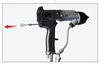
4. Remove air valve packing nut and packing.
