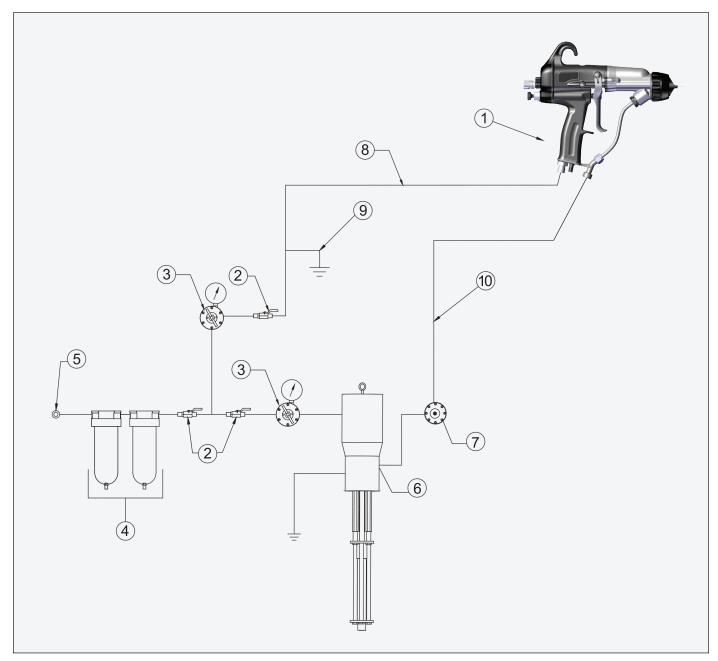
Figure 2: Ransflex Typical Solventborne Installation
