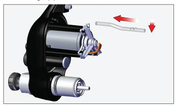
6. Install fluid valve cartridge.
