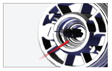
3. Install fluid nozzle using 80353-00 wrench. Tighten till nozzle seats on O-ring and then 1/8 additional turn.
