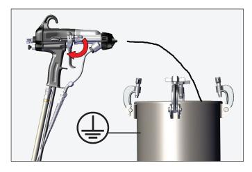
4. Release trigger stop material flow.
