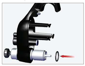
4. Install screw and retainer.
