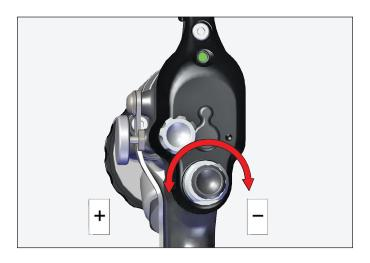
16. Adjust compensation valve with small driver.
