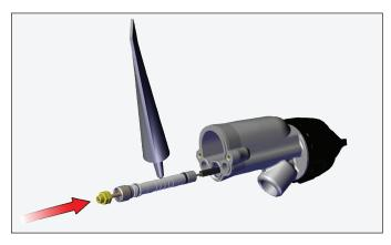
2. Tighten packing using wrench. Pull back and forth on the needle shaft till a slight amount of drag is felt.
