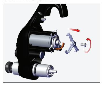
3. Remove motor assembly by pulling out on 3 arms, pull motor out.
