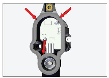
8. Push rear cover assembly into handle and tighten cartridge.
