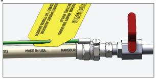
3. Activate trigger to start material stream into **grounded metal bucket or suitable area**.
