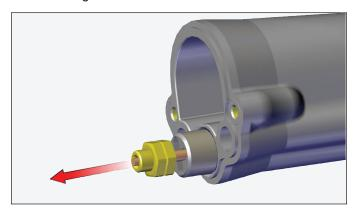
4. Remove jam nuts using 10mm wrench.
