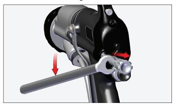
3. Remove rear cover and cartridge with 15mm wrench.
