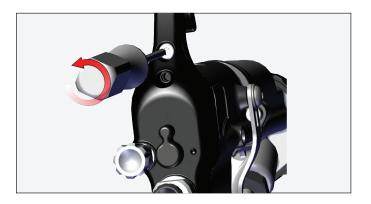
2. Remove fan air cartridge with 10mm wrench.
