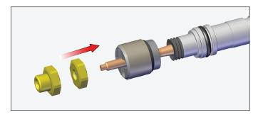
11. Install rear nut. Install jam nuts finger tight.
