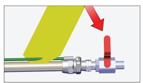
3. Discharge fluid into appropriate earth grounded metal container
