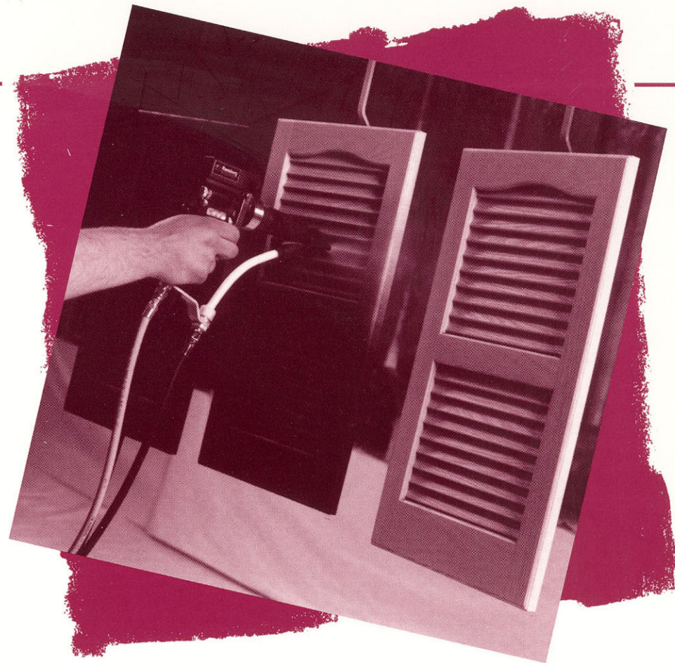
Inability to paint in corners, recesses and plastics is yet another myth about electrostatics.
