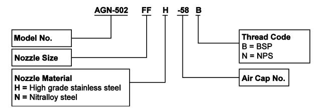
AGN-502 Spray gun fitted with fan air control valve.
