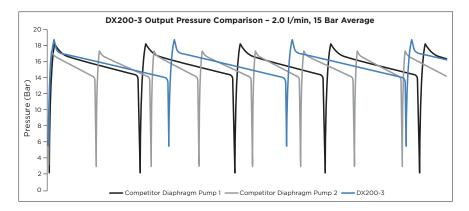
The 'longer—slower' cycle rate of the DX200-3 moves the same volume of fluid but at a slower cycle rate than its competitors. This means less stress and wear on components, resulting in longer intervals between maintenance inspections.
