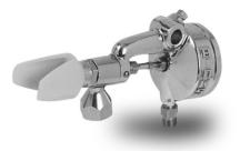
Same as Model 550, but constructed with larger fluid inlet and passages. Used for spraying heavy materials such as mastics and undercoatings. Spray nozzle not included, order separately. (Maximum operating pressure is 3000 PSI.)
